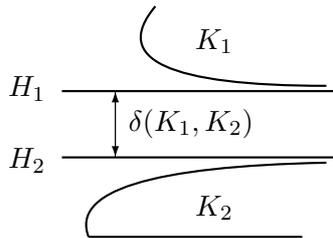
Figure 14: Separation of  $K_1$  and  $K_2$  by a slab of maximum width.
